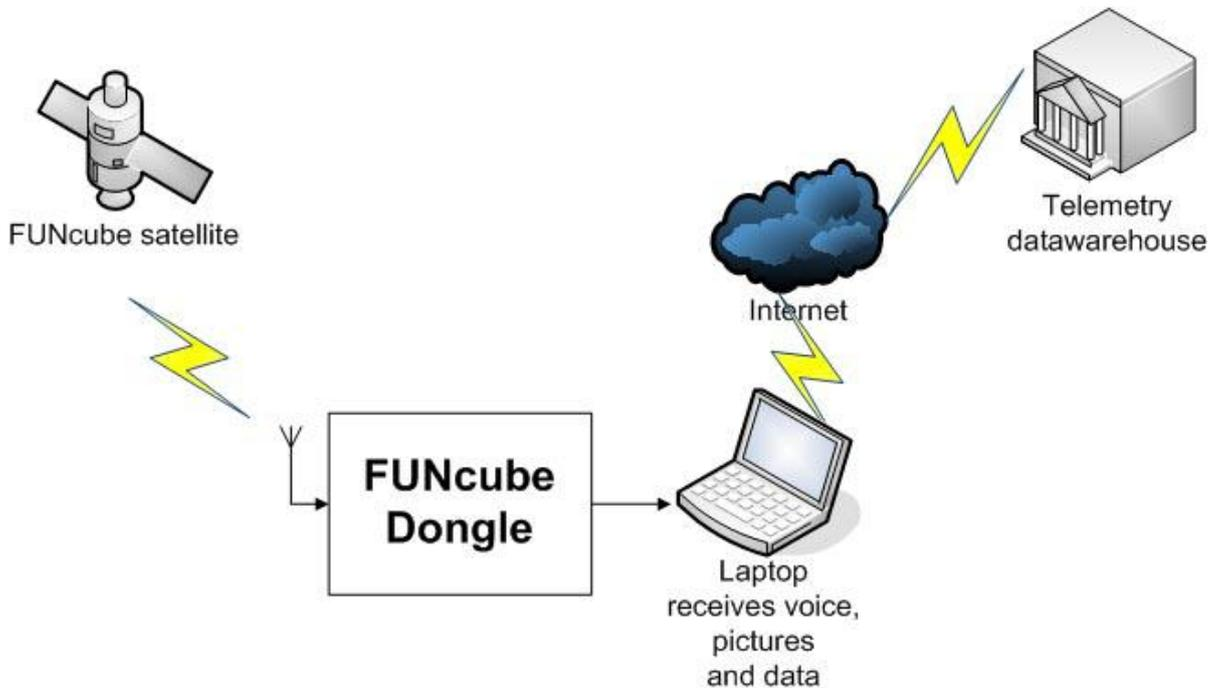
The FUNcube satellite also includes an analogue voice transponder that can also be received with the FUNcube Dongle.
