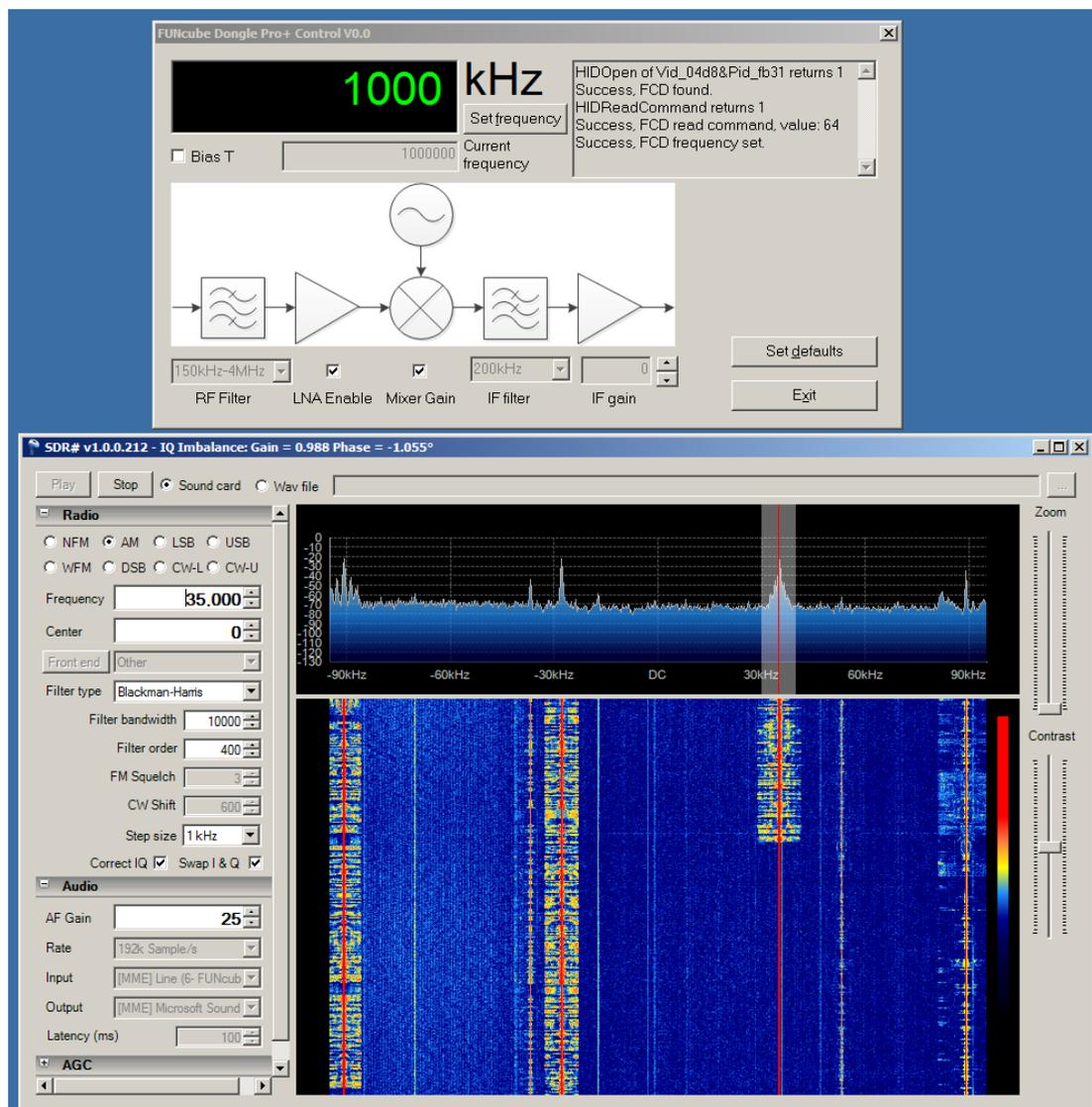
For wideband FM (WFM) signals, almost the entire 192kHz is required for demodulation, and it is recommended that that the demodulation's carrier (the vertical red line) is set to the centre DC position. In this case, the FCHid frequency is the same as the broadcast signal's frequency. In radio terms, this is a single, direct conversion receiver.
